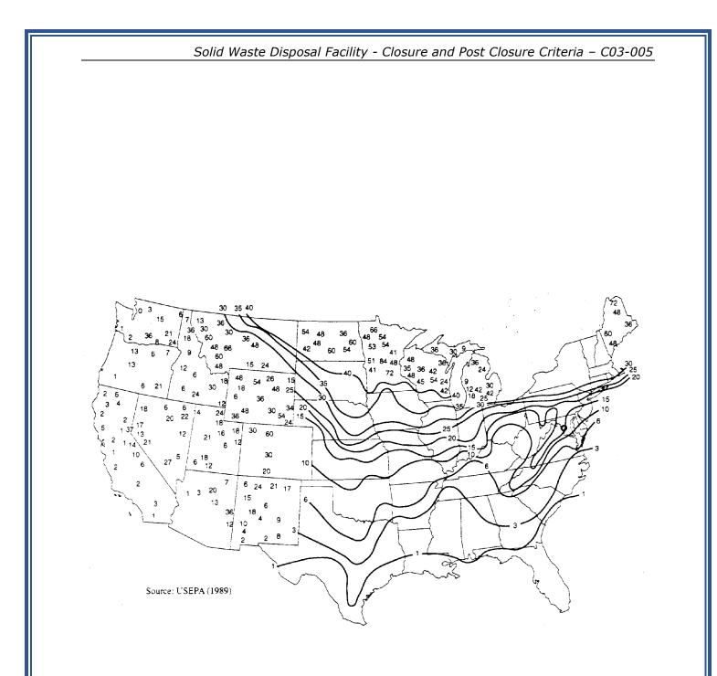
Figure 6-4 Regional Depth of Frost Penetration in Inches
