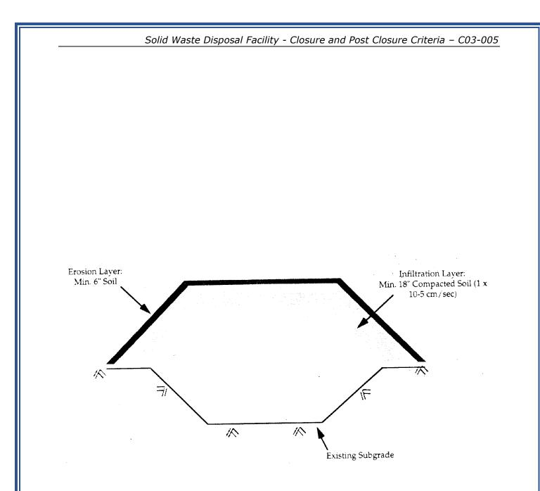
Figure 6-1 Example of Minimum Final Cover Requirements
