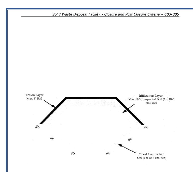
$Figure \ 6-2 \\ Example \ of \ Final \ Cover \ With \ Hydraulic \ Conductivity(K) \leq K \ of \ Liner$
